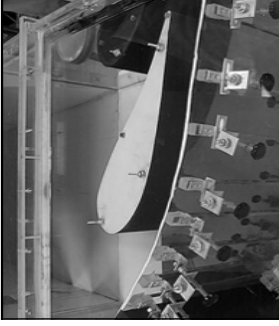
Figure 4. Large-scale turbine vane in wind tunnel.
